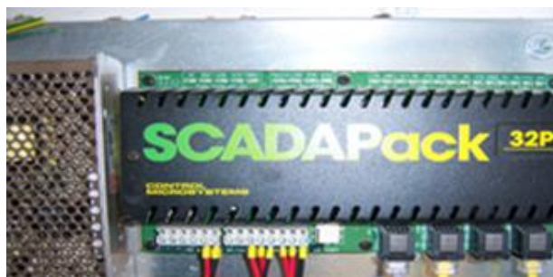
Figure 3. SCADA Pack 32P assembled view
